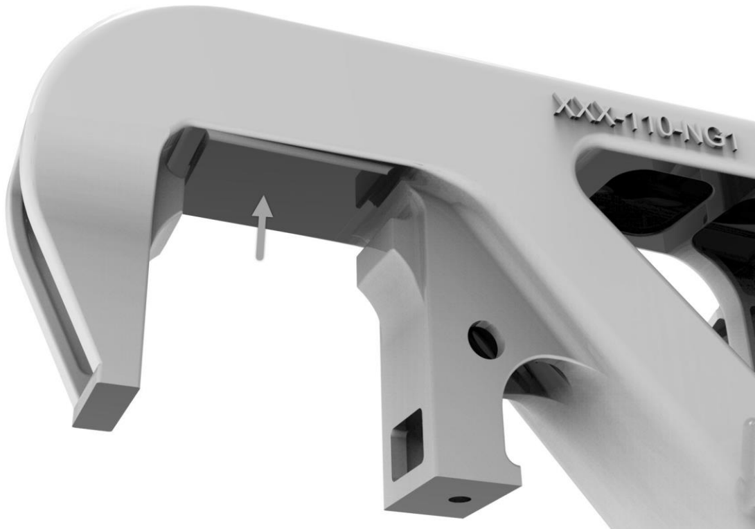
Figure 14: Side Frame Pedestal Roof Wearing Surface
